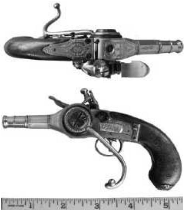
Above: two views of Flintlock self-loader by Andrew Dyson. Note the belt loop, nice engraving, and wire inlaid stock. OAL 5.5"
