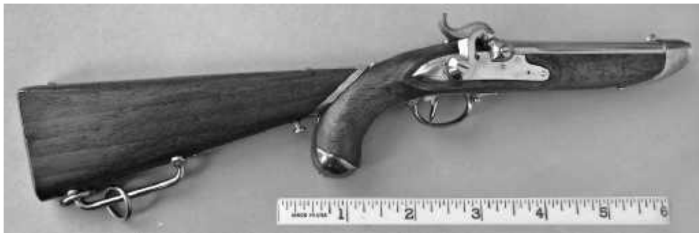
Below: 2/5 scale Model 1817 German Percussion pistol - Converted from Flintlock - with shoulder stock made by G. Ball. OAL pistol 5-7/8" with stock OAL 10"
