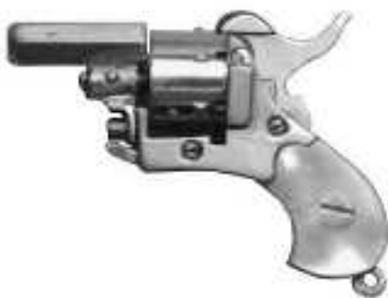
Above, an enlarged view of the left side with the trigger in the folded up position.
