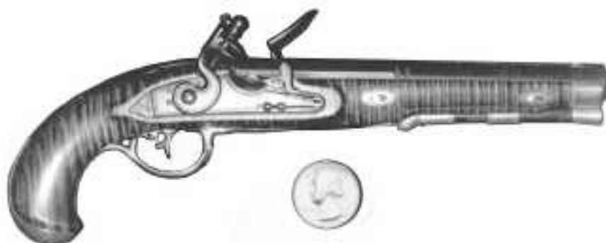
Above; a pair of 1/4 scale, early American, flintlocks. OAL 5" With ivory grips, steel barrel and lock, and a nicely engraved silver butt plate.
